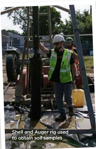
Shell and Auger rig used to obtain soil samples
